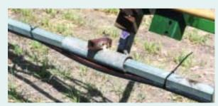
This weed wiper uses recycled-rubber, porous hose instead of a rope wick to apply chemical. The choice of chemical is limited as some rapidly destroy the porous hose. Gravity, rather than a pump, is used to move chemical along the hose.
