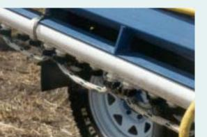
A purpose built broad-acre wick wiper fitted with rope wicks, seven individually controlled sections, and hydraulic height adjustment.
