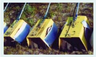
Both types of shields have thick curtains slit vertically to reduce spray escape from the rear corners of the shield into the base of the crop. Photos: Mike Collins
