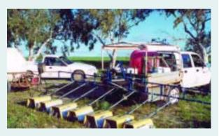
This system consists of a 7 shield sprayer for an 8 row trial combine. Row spacing was 65 cm. The grower is making up a light, 4WD bike towed spray trailer for use in lupins.
