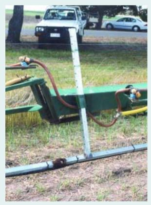
A simple bracket holds the bar and porous hose and can be adjusted to various heights above the ground.
